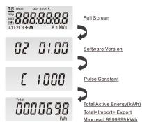
After the self-checking program, the meter display will show the total active energy (kWh)  $% \left( \frac{1}{2}\right) =0$
